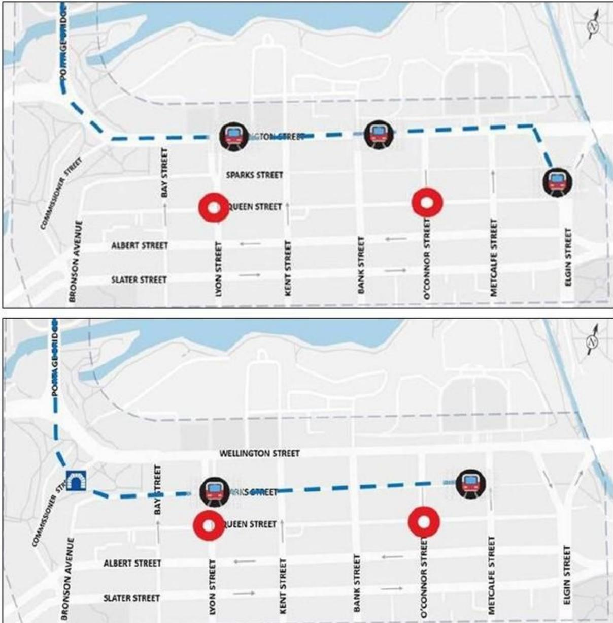
Figure 1: Top: Tramway corridor options on Wellington Street (surface) and Bottom: Sparks Street (tunnel)
